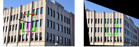
Figure 2. Geometry from a low-rank patch on a building facade. Left: The red box represents the selected candidate region I , and the green box corresponds to the recovered low-rank texture using TILT. Right: The rectified building facade I_0 = I \circ \tau using the homography \tau estimated from the low-rank texture.
