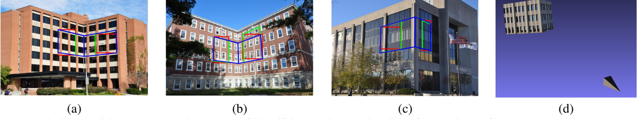
Figure 4. (a)–(c): Additional representative results of identifying the intersection line of two adjacent facades. Red windows are the initialization. (d): Accurate 3D ‘pop-up’ from the single image in Figure 3. Camera position is recovered, shown as a small pyramid.
