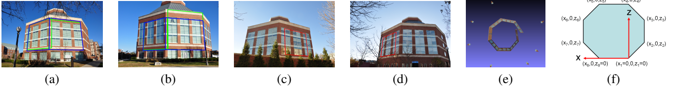
Figure 9. (a) and (b): Segmentation (green) and intersection detection (blue) on two images of an octagonal building. (c) and (d): A pair of matched regions from the same facade with different partial occlusion. (e): A top view of the reconstructed structures of the octagonal building showing the accumulated geometry error when assembling the views one by one. (f): The parameterized 3D model of the building.
