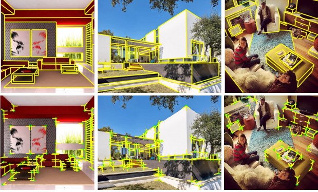
Figure 2. Example images of our wireframe dataset, which covers a wide range of man-made scenes with different viewpoints, lighting conditions, and styles. For each image, we show the manually labelled line segments (first row) and the ground truth junctions derived from the line segments (second row).
