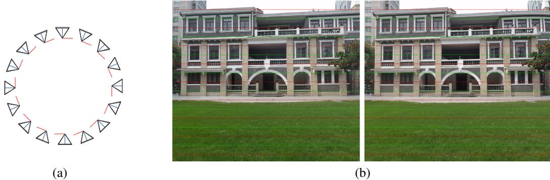
Figure 5. Visualization of the results with calibration targets. **(a)** The relative positions of the 16 cameras estimated by our method. The top camera is the reference camera. **(b)** An example rectification results for two of the cameras using the estimated extrinsic parameters.
