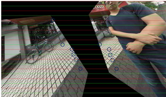
Figure 8. Rectified street view images with the estimated extrinsic parameters. We have marked some areas with blue circles for easy inspection of the vertical parallax between the two rectified images.
